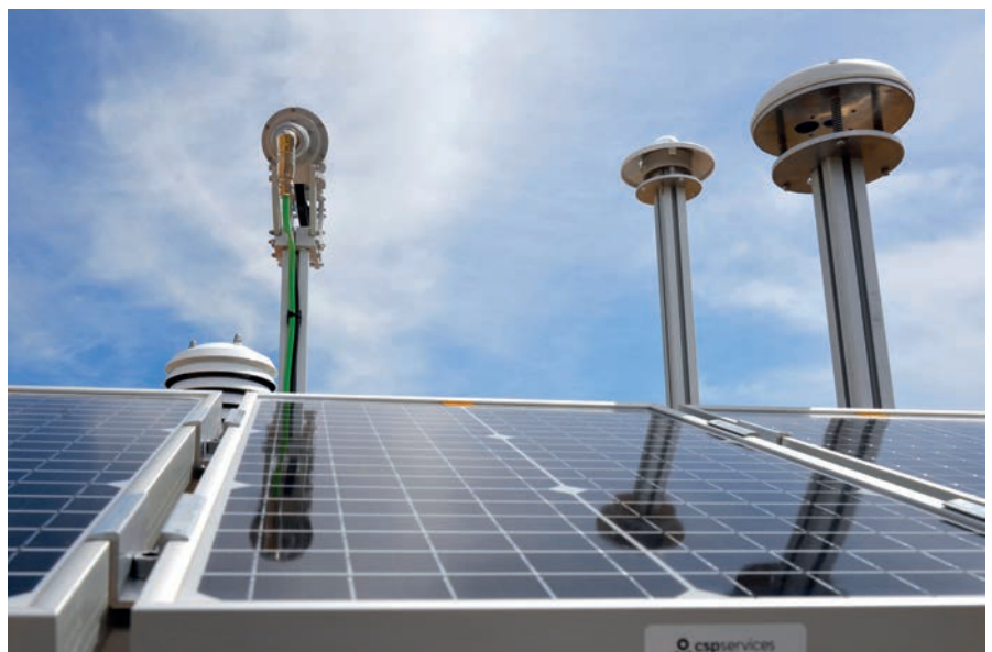
Cloud camera combined with other weather sensors
