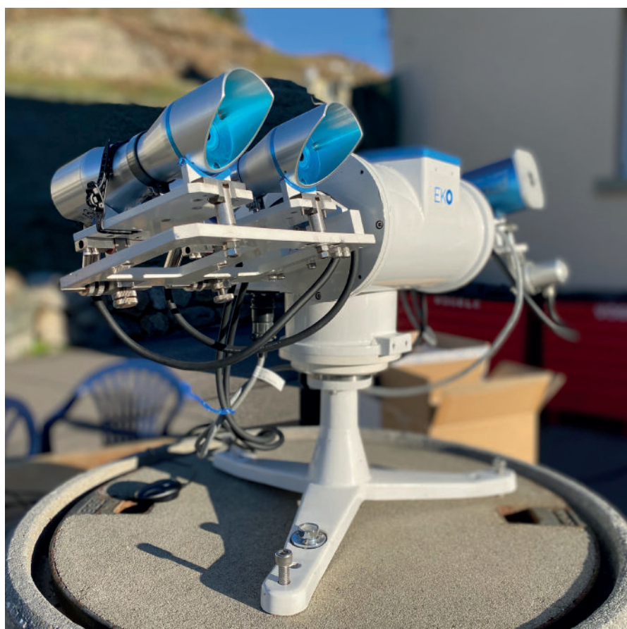
STR-22G Sun Tracker & MS-57 Pyrheliometers at IPC 2021 in Davos, Switzerland
