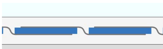
Fig. 1: Structure of a conventional solar module with connector, or wire-connected solar cells. © M10 Solar Equipment GmbH
