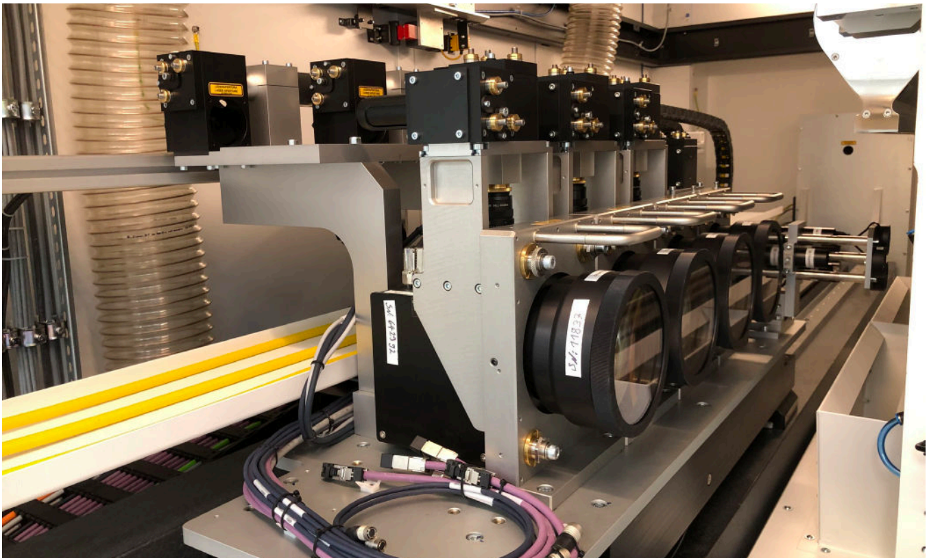
Fig. 3: Cross-web stage of P2/P3 tool with four scan heads and cameras
