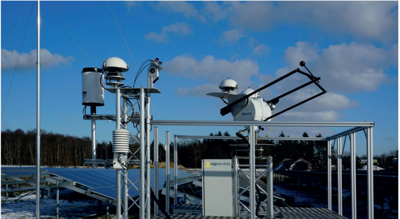
Automatic weather station with integrated cloud camera for nowcasting
