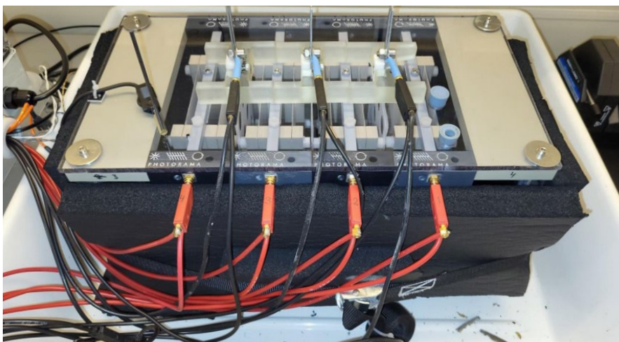
Electrowinning cell for Ag production at SINTEF
