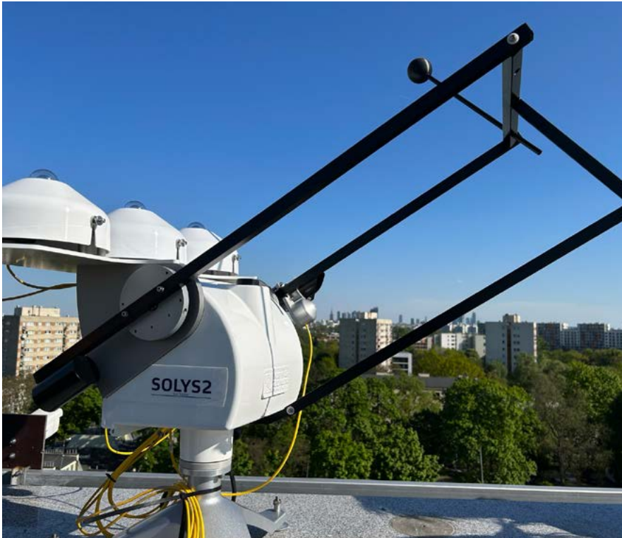
Kipp & Zonen ventilation units can be easily mounted on pyranometers, pyrgeometers, and UV radiometers. This image shows a Kipp & Zonen SOLYS2 sun tracker being installed at the Polish Meteorological and Hydrological Office in Warsaw
