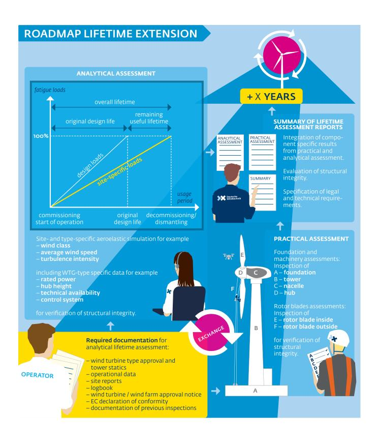
In addition to the complexity of the terrain, consideration must also be given to neighbouring wind turbines, existing infrastructure and effects within the wind farm, with regard to the respective IEC classification (IEC 61400-1: design requirements). In order to ensure efficient verification, it is essential to include
