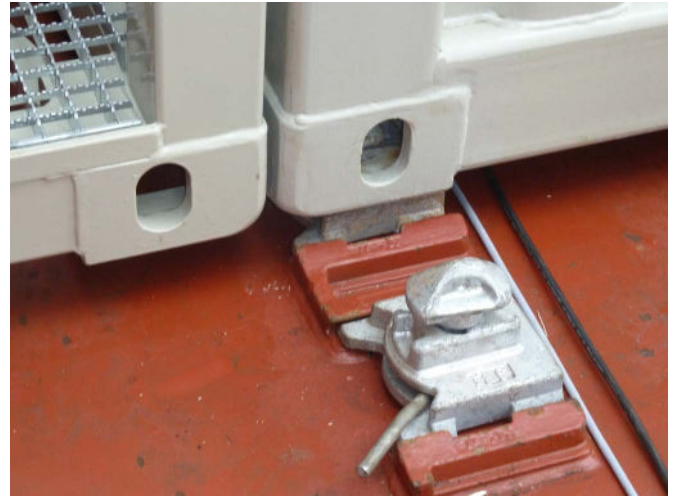
Container easily mounted through twistlocks
