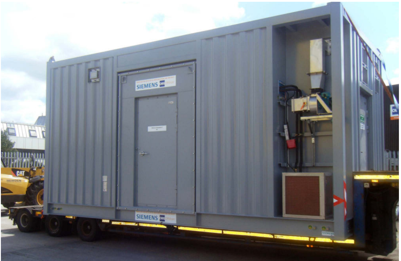
OEG Offshore's custom-built Local Equipment Room (LER) modules for the London Array Offshore Wind Farm
