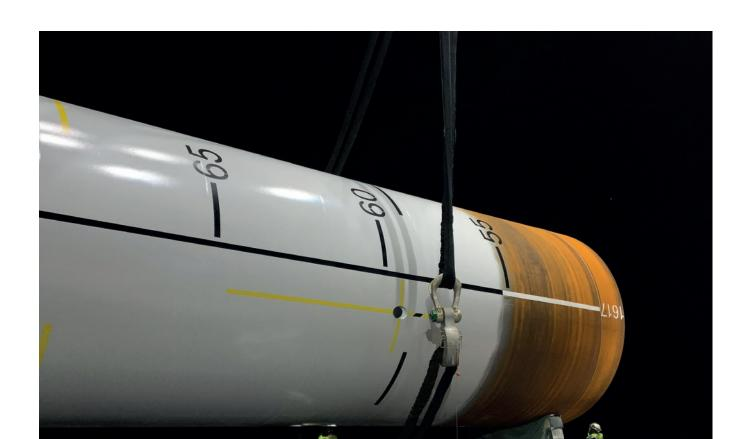
requiring 28 monopiles in total. The substation monopile, which is one of the first to be transported, weighs just over 2,100 tonnes, has a length of 110 metres and a diameter of 9,60 metres, making it one of the biggest monopiles in offshore wind history and the biggest in Europe.
