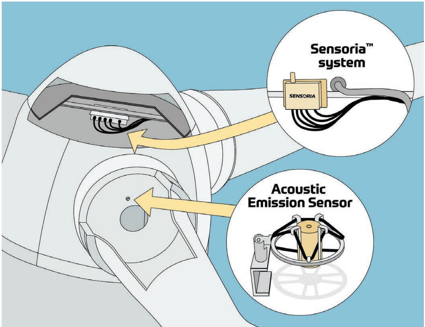
Permanently-installed sensors in blades reduce the need for in-person inspections by detecting defect activity in real time
