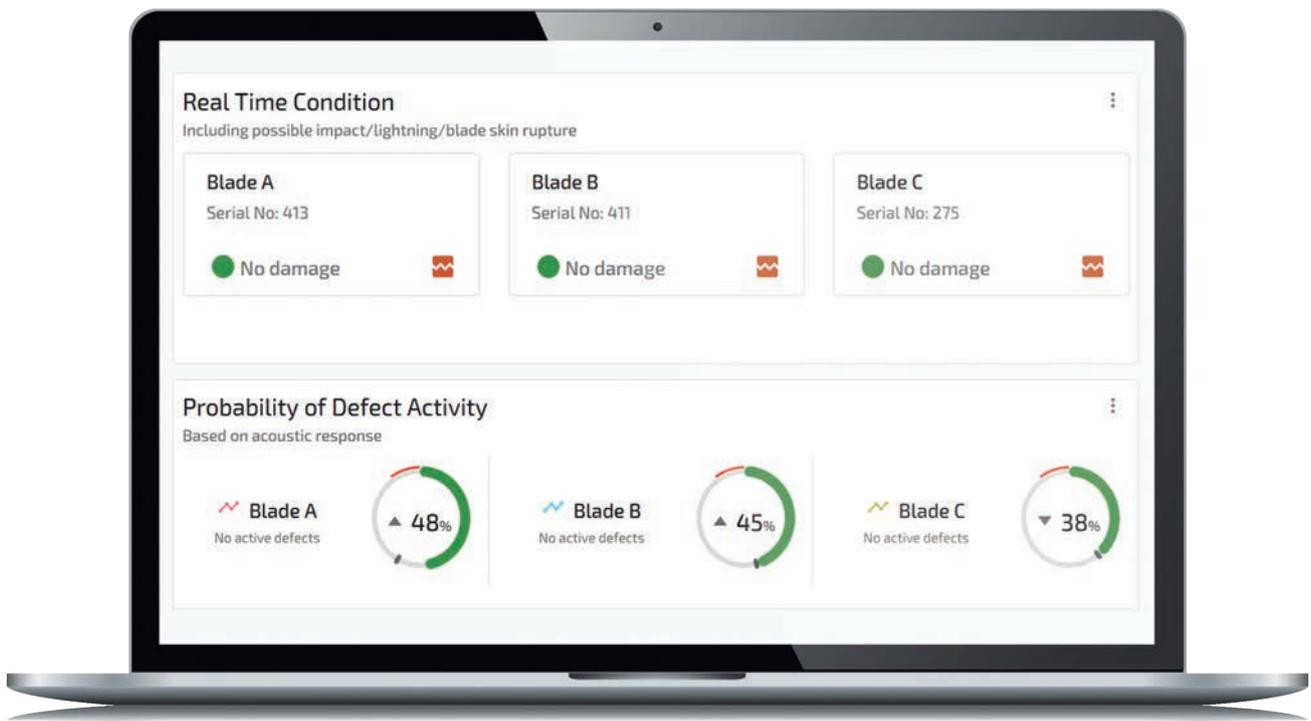
The Sensoria Insights data portal enables operators to prioritize blades for inspection by visualizing blade integrity data and alerting personnel to potential concerns
