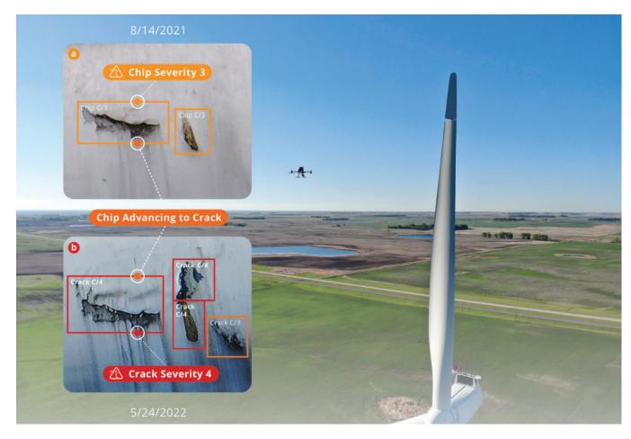
the necessary follow-up activities after an operational event, which can lead to additional costs and labor. For example, some blade models are particularly vulnerable to off-receptor strikes from lightning and require an internal inspection to check the spar bond joint. This can be confirmed by drone before full inspection.
