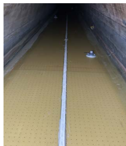
Figure 1: Shape sensor installed in a blade
