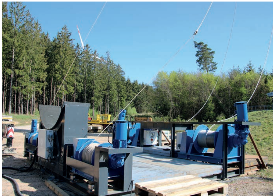
The GBWS support frame can be used immediately thanks to pre-assembly
