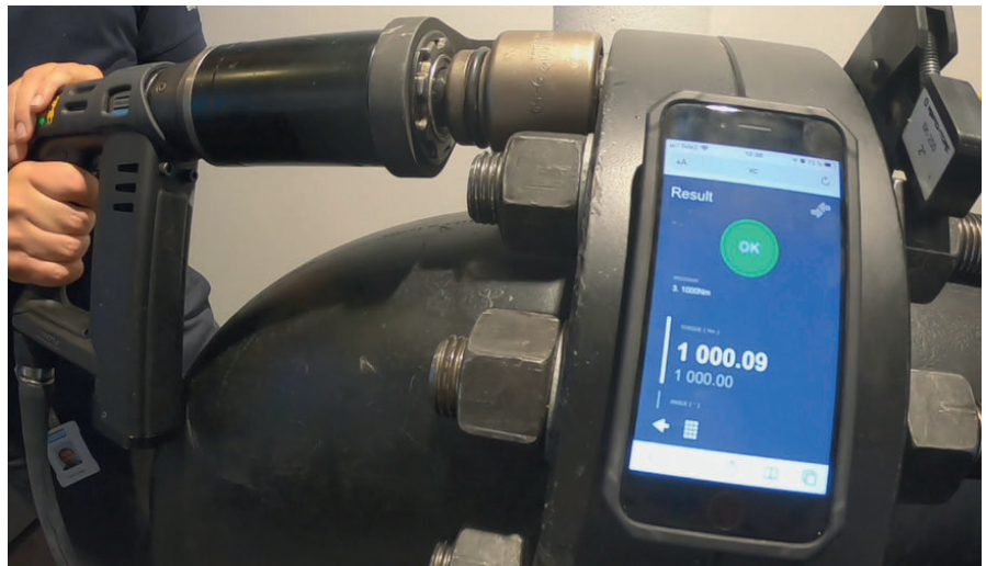
Tools connect to 'any smart device' so no need for complex and costly control panels.
