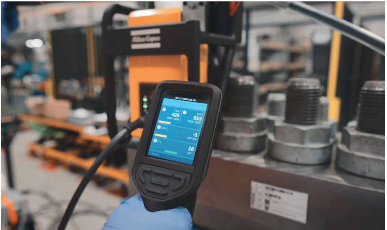
Visual feedback on tools and devices ensures that the operator gets feedback without need for external devices or gauges.
