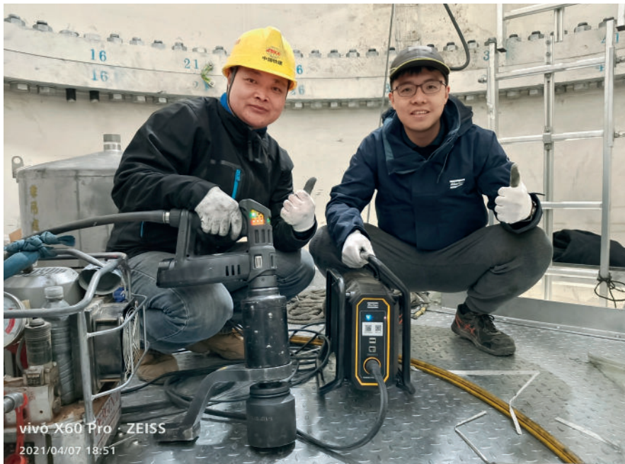
Tensor Revo nutrunners can reduce bolting process time by more than 50%
