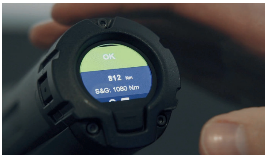
Feedback on tightening status allows operators to address problems at source so that processes can be completed right first time.
