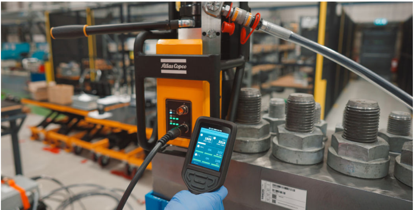
The Smart Tensioning System has a hand controller to guide the operator, which speeds up the process, reduces the risk of errors whilst always securing safe operation
