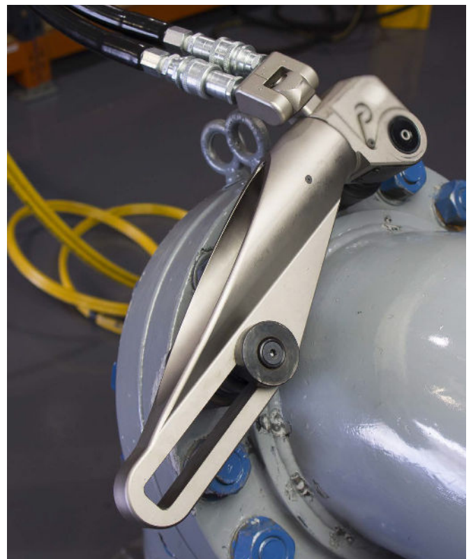
A sliding drive reaction bar with a socket on an adjacent nut with no risk of finger or hand injury
