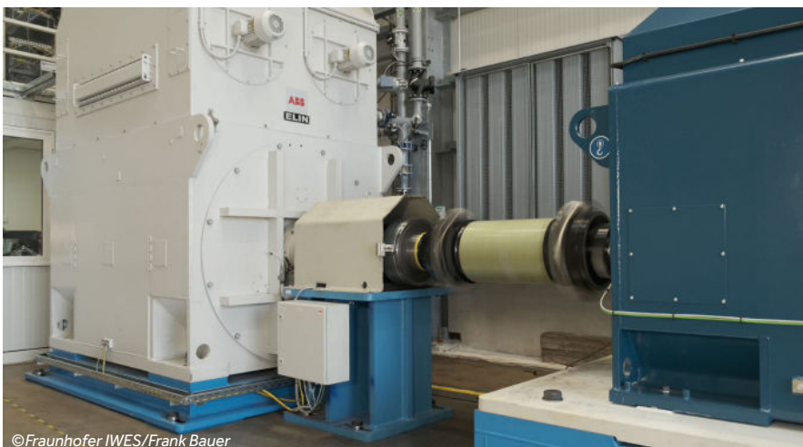
The 9 MW drive motor of the HiL-GridCoP test bench
