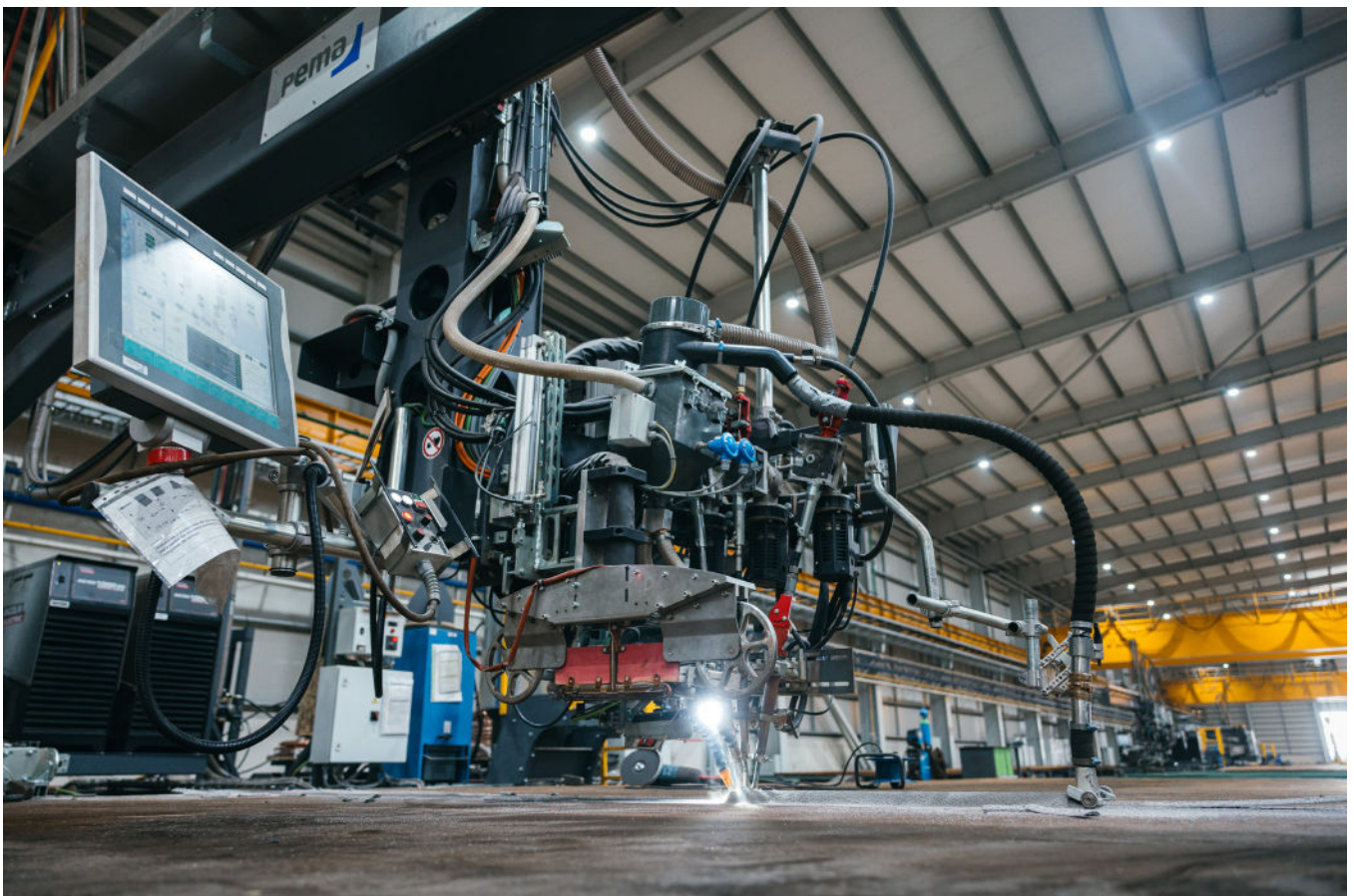
The triple long stick-out process, combined with PEMA WeldControl and robust handling systems, delivers proven performance and quality gains in large, thick structure welding
