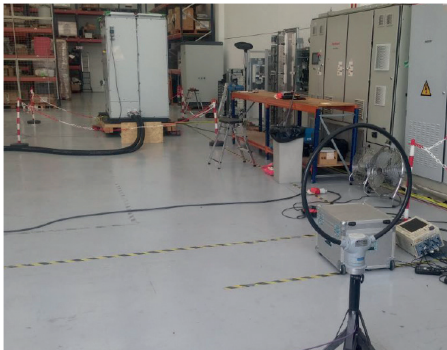
Figure 9: Radiated emissions test
