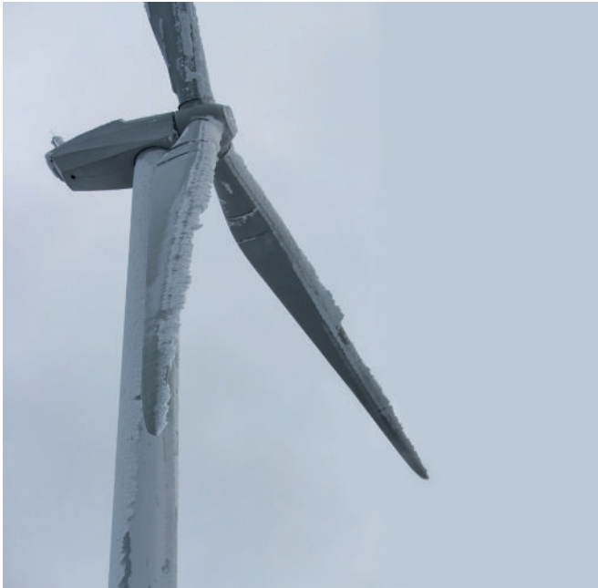
These photos were taken on the same day. The turbine on the left is without any blade heating. The turbines on the right have retrofit blade heating and thus, aerodynamically critical areas are free of ice and snow.
