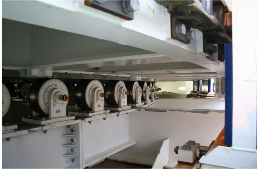
process two products simultaneously, or a single length of product up to 10,000Te. This minimises offshore jointing requirements which is a significant advantage, technically and commercially. The company was responsible for the design of the full lay spread for the vessel, including a 75Te capstan to compliment the five tensioners of varying capacities, as well as stern mounted lay wheels and two carousel mounted spooling arms.
