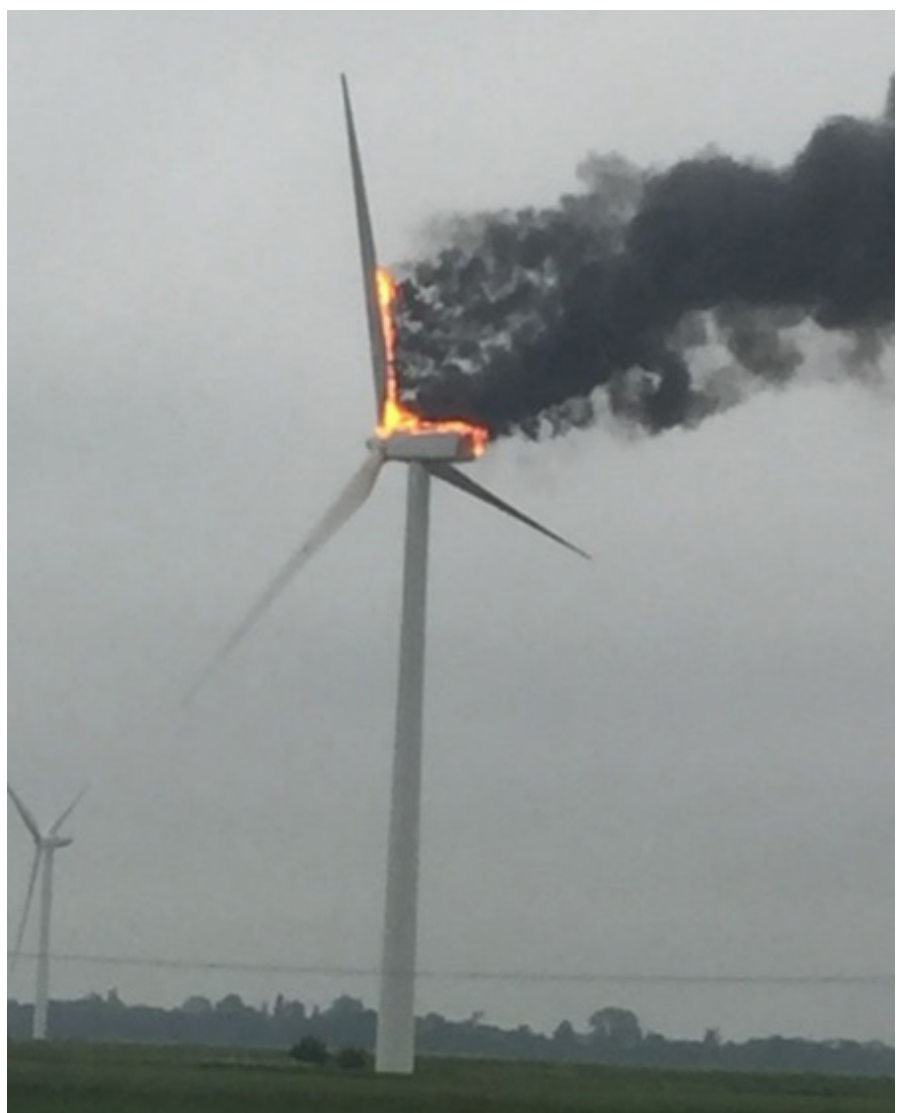
Figure 3: A recent wind turbine failure due to a lightning strike in Crowell TX. Photo credit Brent Havins
