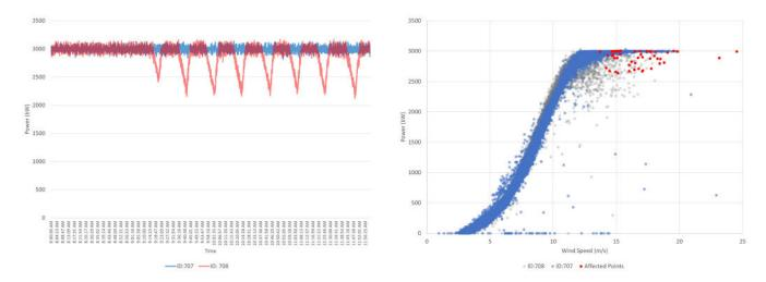
Turbine exhibits significant and frequent reductions in power, but the power curve does not highlight the magnitude of these events
