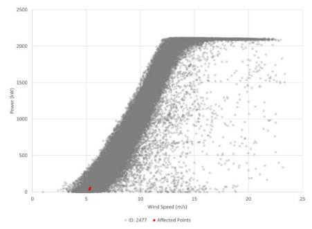
Turbine is continuously trying to start, but fails because it does not reach a sufficient generator speed in time. Over 100,000 startups aborted per year at the farm, but no significant power curve behavior was observed
