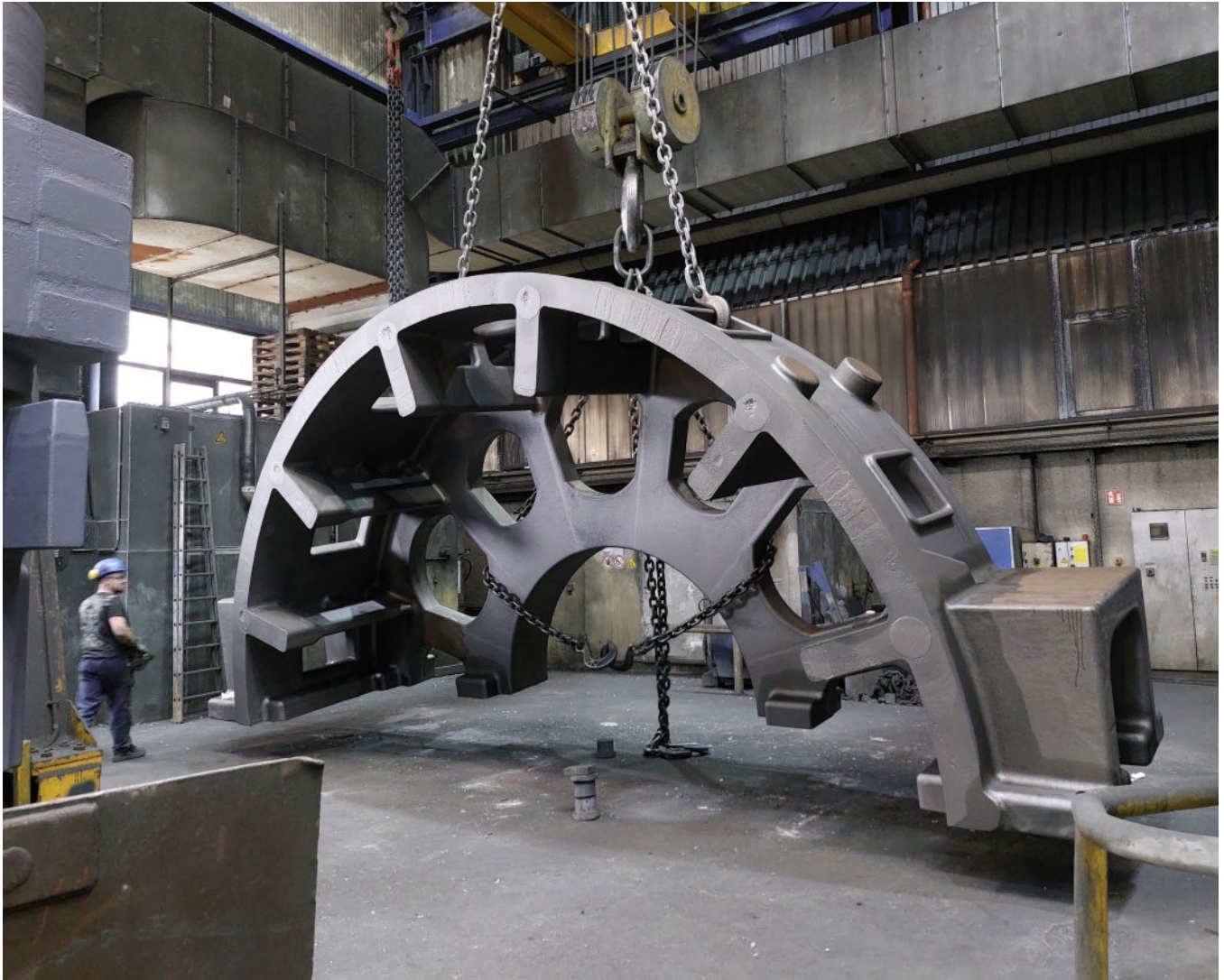
Casting of the upper half of the housing of the 35 MW multi-motor drive system
