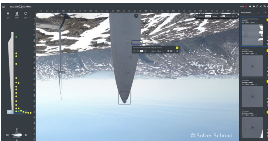
Damage annotation in 3DX™ Blade Platform
