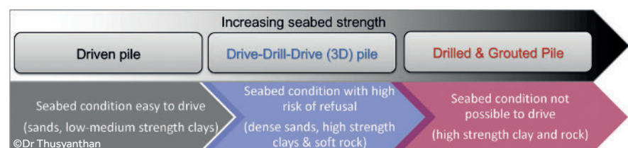
Figure 5. Recommended pile installation methods based on seabed condition
