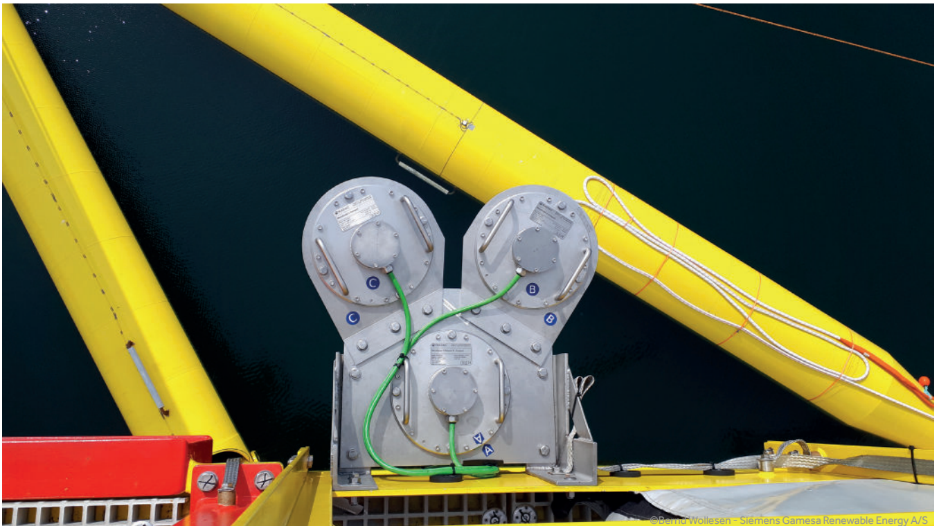
Radac wave radar (WaveGuide 2 Direction Onboard 2) installed on the floating TetraSpar turbine
