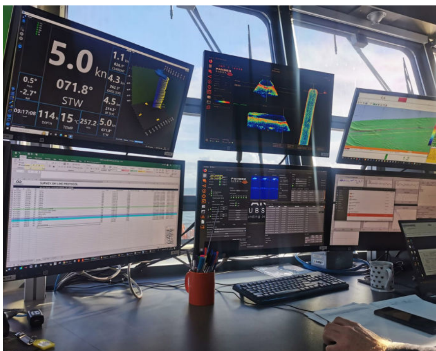
The Nortek VM Operations provides real-time oceanographic data, as seen here in the monitor top left, to the bridge and survey rooms, where it is most needed offshore
