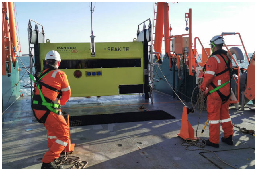
The Kraken Robotics SeaKite Sub-Bottom Imager was towed behind the Geo Ranger to perform the sub-seabed survey
