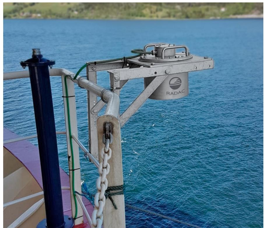
field experiment. This involved a comparison between data gathered from a Directional Waverider buoy and data obtained from the WaveGuide. This comparative study took place at Prinses Amaliwindpark, situated 25 kilometres off the Dutch coast. Over the course of several months, two variations of the Directional WaveGuide were evaluated alongside a Directional Waverider.
